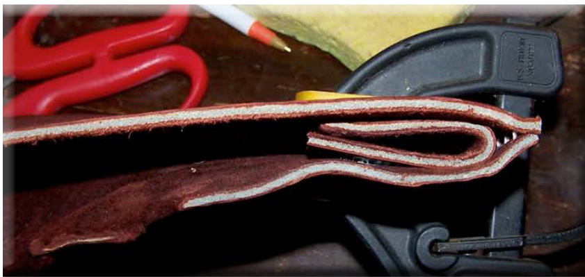
Figure 3: Side view of the reinforcement of the bottom seam to protect the seam from damage by arrow tips.
