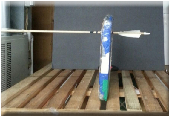
Figure 1: Target area too soft, arrows blowing through.
